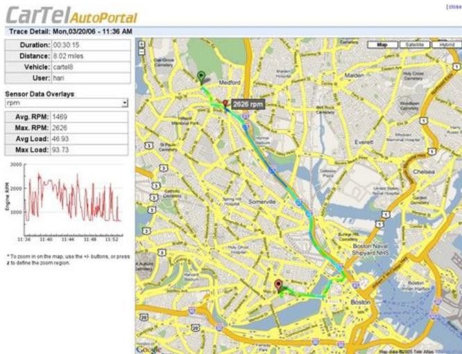
Figure 2. Screenshot of the AutoPortal prototype. Here, the user is visualizing a recently driven route.
